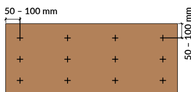
GUTEX Thermoroom® 20 mm; 12 cramps/screws per board
