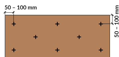
GUTEX Thermoroom® 40 - 100 mm; 8 cramps/screws per board
