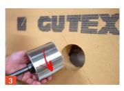
Release ejector by turning the blade.
